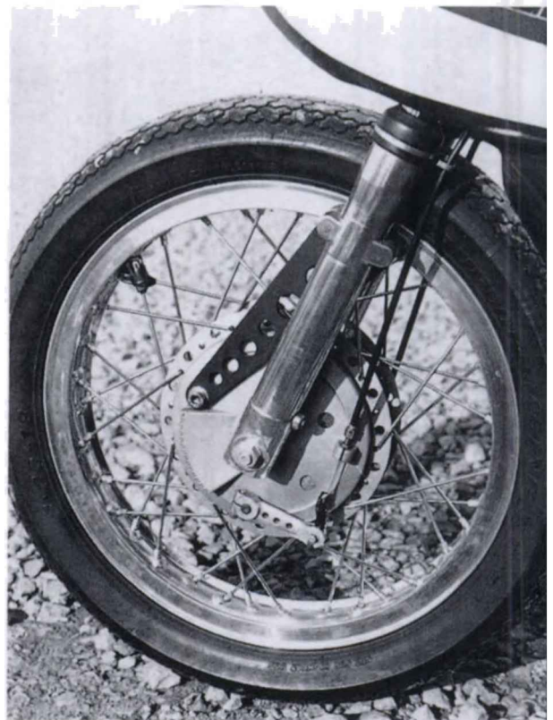
The double-sided, single-leading-shoe Grimeca front hub first appeared on the Mark 3 and Desmo models in 1972. Its power and smoothness make it an attractive choice with classic racing enthusiasts
