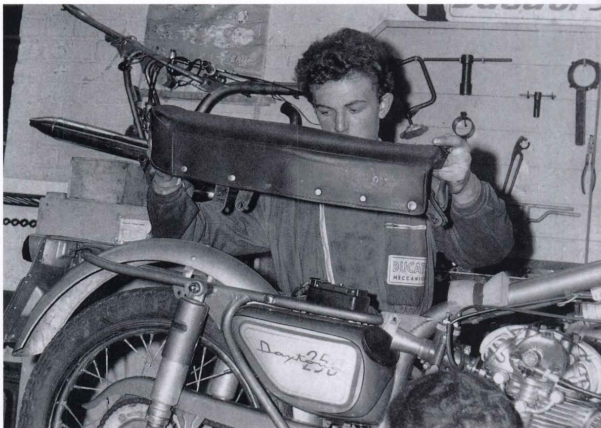
ABOVE Slightly larger than the 175 Sport seat, and with a little more padding, is this seat fitted to the European 250 Diana (Daytona in Britain) of 1962
