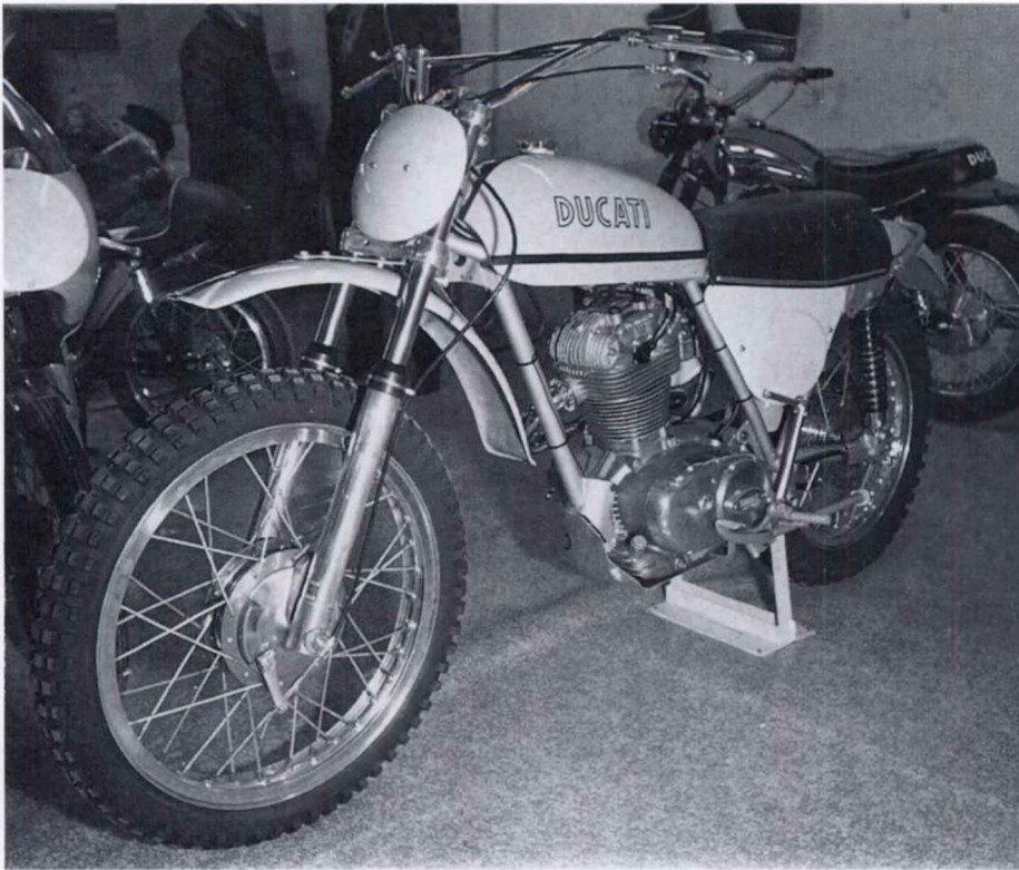
LEFT The 450 R/T Desmo (1971-2) has a purpose-built frame which owes very little to the series-production roadster chassis. It was largely intended for Stateside off-road use
