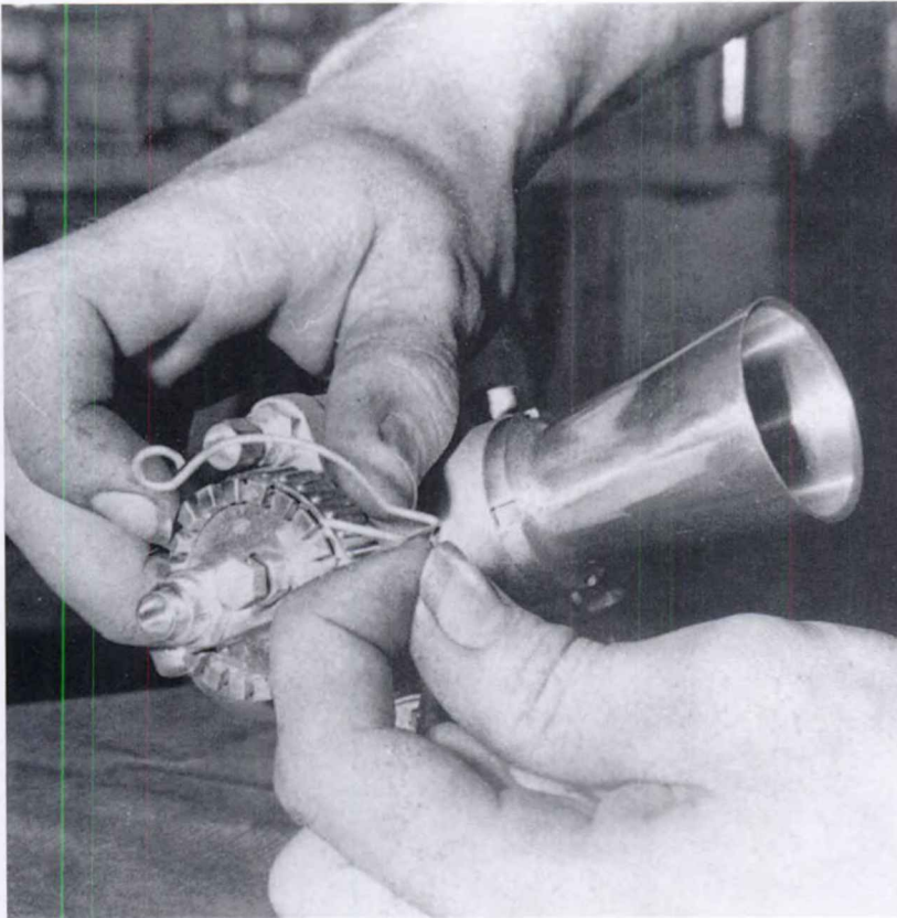
The slide/mixing chamber cover is held securely in position by this special spring. It must be removed before unscrewing the cover
