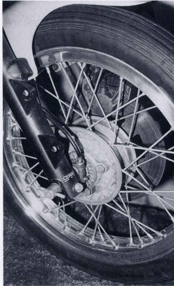
The disc brake hub is the same component as that fitted to the wire-wheel 900SS and certain other early V-twin models. It has 40 spokes
