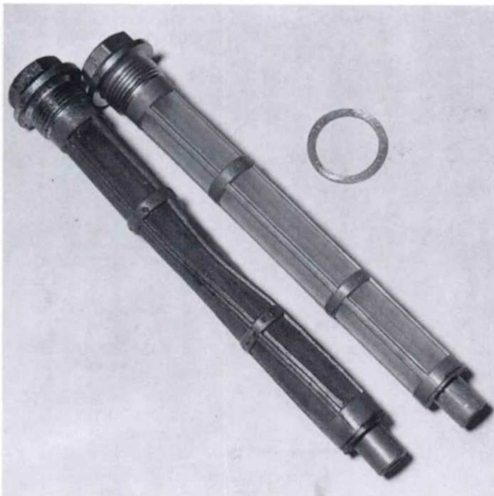
The nylon gauze sump filter can easily become damaged if the end (nose) section is not located correctly into the opposite side of the crankcase. A new filter and alloy gasket are shown on the right
