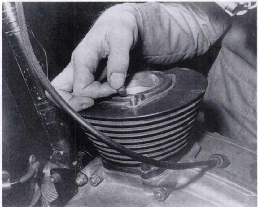
Always make sure that a new head O-ring is fitted each time the head/ barrel joint is disturbed
