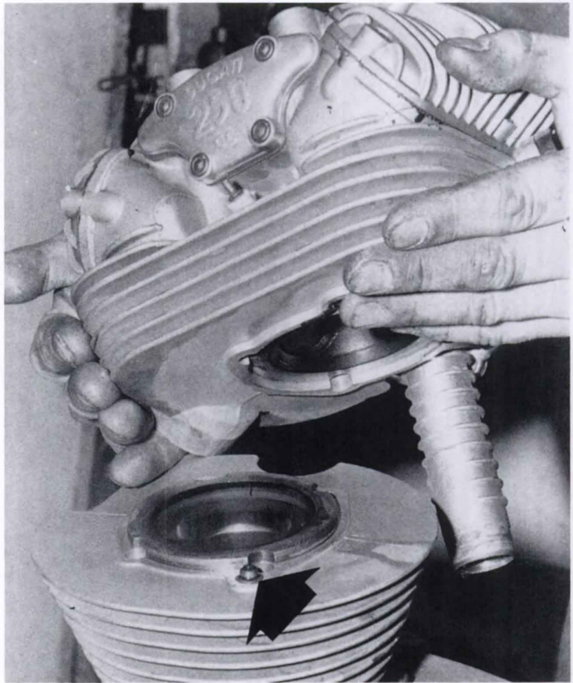
There is no cylinder head gasket, only a rubber O-ring (shown)
