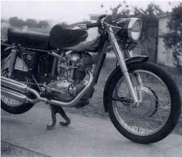
Early models, such as the 175 Sport and 200 Elite (shown), originally had this branched exhaust pipe and double-barrel silencer. It provided poor cornering clearance, however, so most owners soon ditched the system in favour of a single Silentium
