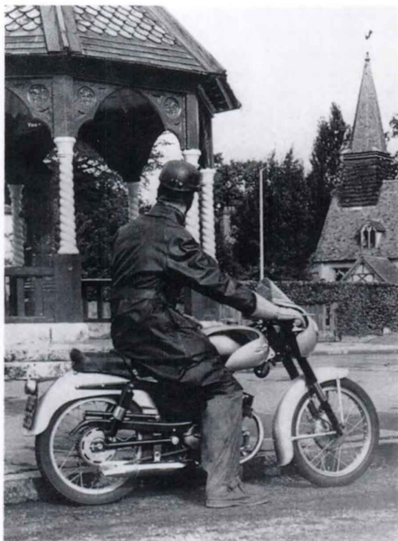
LEFT By 1956 the 98 Sport wore a small handlebar-mounted fairing. This particular machine is under test with the British magazine Motor Cycling
