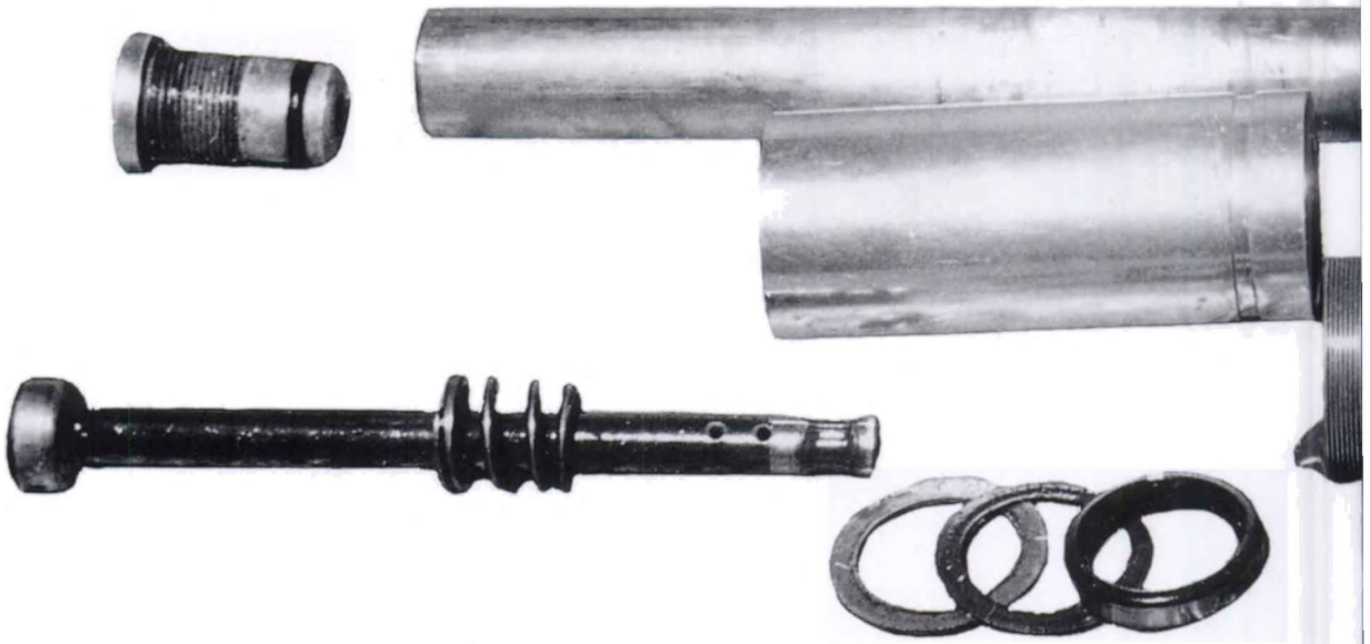
ABOVE Some of the component parts from the 31.5 mm forks, including stanchion, slider, valve assembly, fork top alloy plug, oil seal and washers
