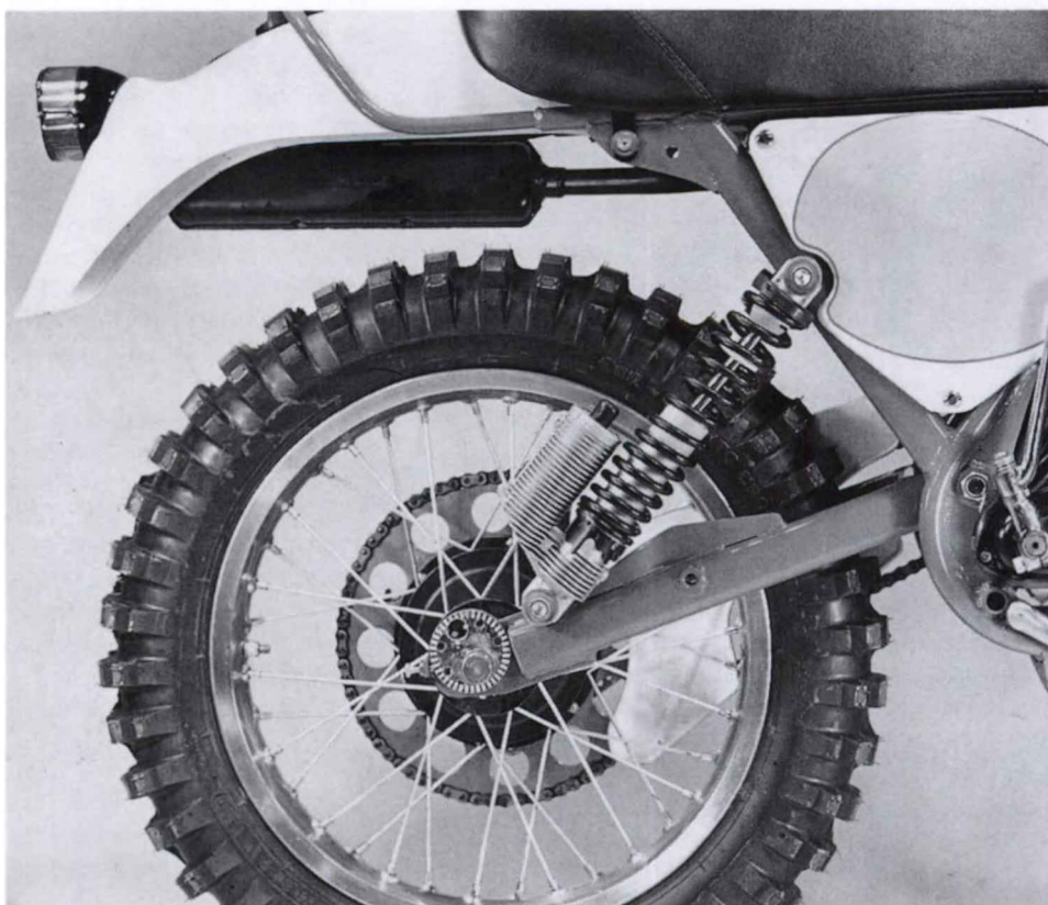
Unique to the 1977 125 Six Days enduro is this option of mounting the rear shocks vertically or at an angle. The finned cylinder is a gas reservoir
