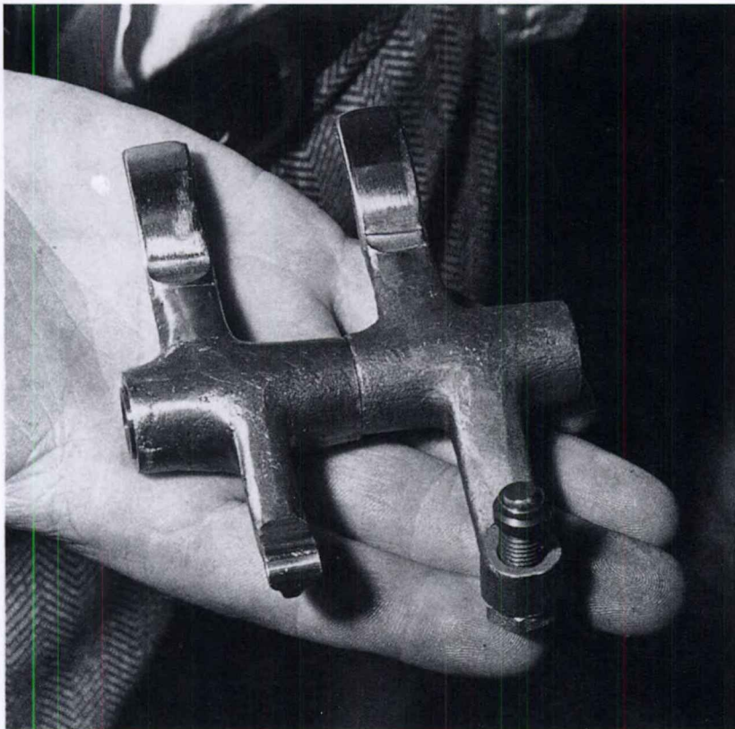
Two types of Ducati rocker: solid (shim type) on the left, conventional adjuster and lock-nut variety on the right
