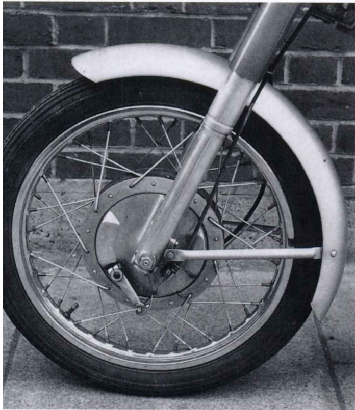
The 180 mm single-leading-shoe front brake fitted to all ohc singles of 175 cc and above, from 1957 until the end of 1971. Pre-1965 hubs have seven fins between the spoke flanges, but thereafter this number was reduced to only three
