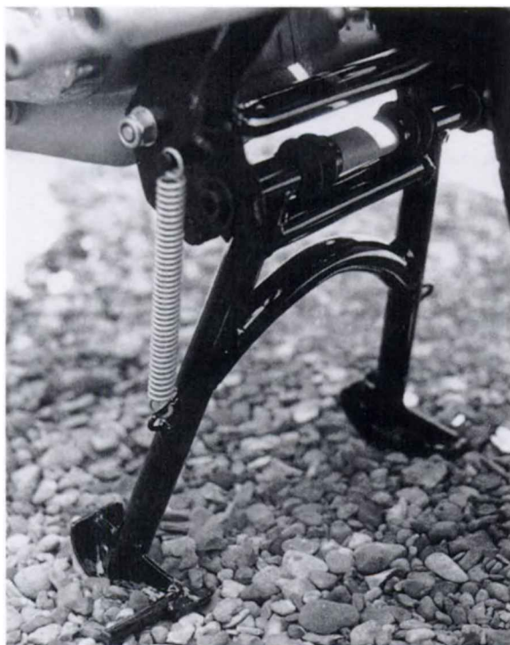
The centre stand fitted to widecase, four-stroke, camshaft models. Both spring and pivot rod are longer than those on other types
