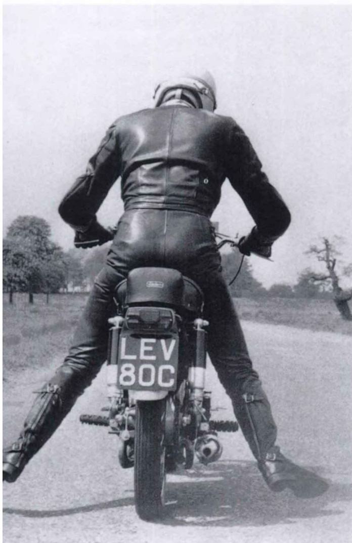
ABOVE Rear number plate, plate holder and rear light. The machine is a 1964 five-speed 250 GT being put through its paces in June 1965
