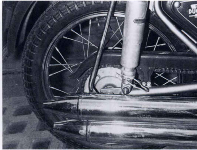
Close-up of the twin silencers. Note Marzocchi-made rear shock with polished alloy top and bottom spring covers
